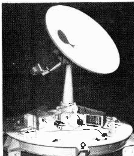
Antenna unit of the Arion shipborne satellite communication terminal from Marconi. Arion, which is the first British commercial marine satellite terminal, made its debut at Communications 76 and is designed to work into the Marisat satellite system. The terminal provides duplex real-time telephony and telex and is capable of carrying facsimile and up to 4,800bits/s two-way data.
